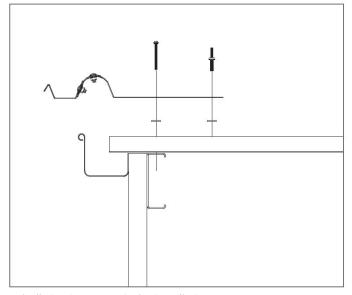
• Fix to roof deck using 6 fixings (combination of 14G tek screw and 8mm bulbtite rivets to suit the installation).
