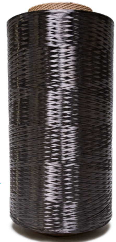
An example of a typical spool of carbon fibre reinforcement fabric used in the process.
